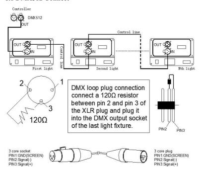
1.In order to reduce signal errors and avoid signal weakening or interference during transmission, a  $120\Omega$  resistance loop can be inserted between the 2 cores and the 3 cores of the DMX output terminal of the last machine.
