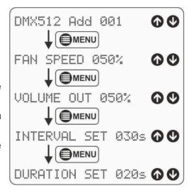
**E.[DURATION SET xxxs]** press the  $\triangle/\nabla$ -buttons (13+14) to adjust the fog duration time (10s $\rightarrow$ 100s) while the fogger is used in timer mode.
